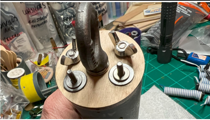
Here's an example of a pair of terminals on a 54mm air frame rocket (fasteners removed from posts)
