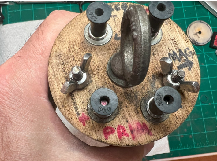
And here's an example of a 75mm Level 3 rocket's redundant drogue circuit e-match terminal sets, with a pair of primary and secondary terminals corresponding to two separate dual deployment altimeters and batteries
