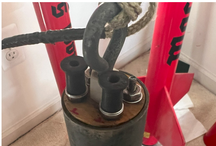
Here's an example of a single set of squib-friendly, e-match terminals for a very slender 38mm rocket
