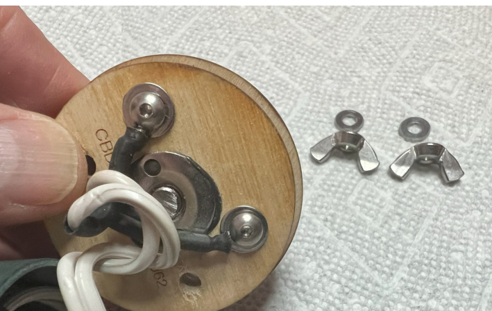
On the reverse side of the bulkhead mounting the e-match terminals, the heads of the posts are wired to the appropriate connectors on the altimeter
