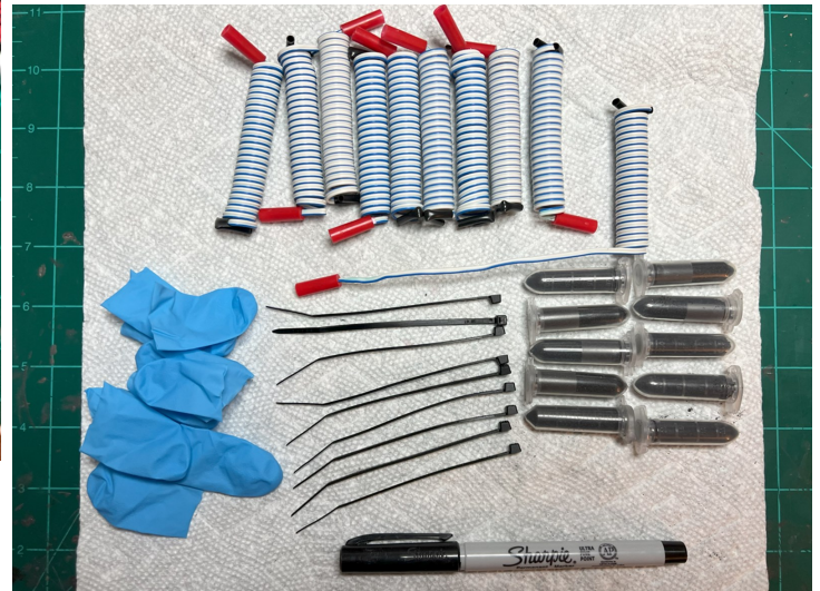
And here's an example of a 75mm Level 3 rocket's redundant drogue circuit e-match terminal sets, with a pair of primary and secondary terminals corresponding to two separate dual deployment altimeters and batteries
