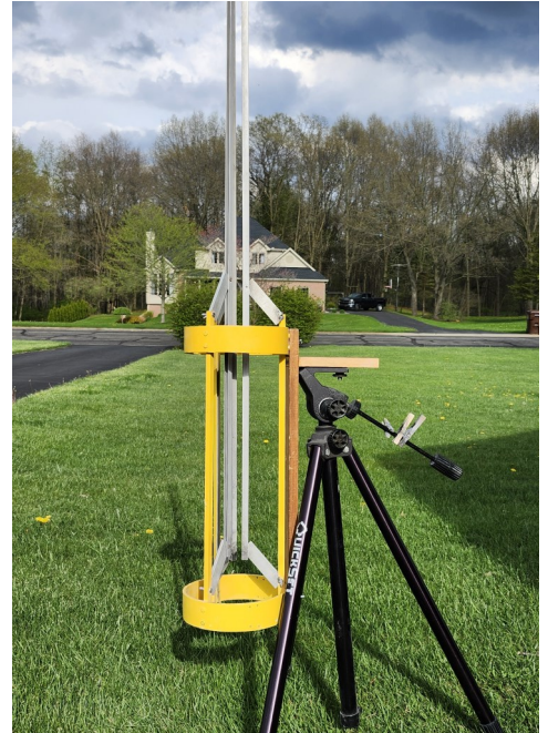
Launch tower made primarily from PVC and aluminum "U" channel
