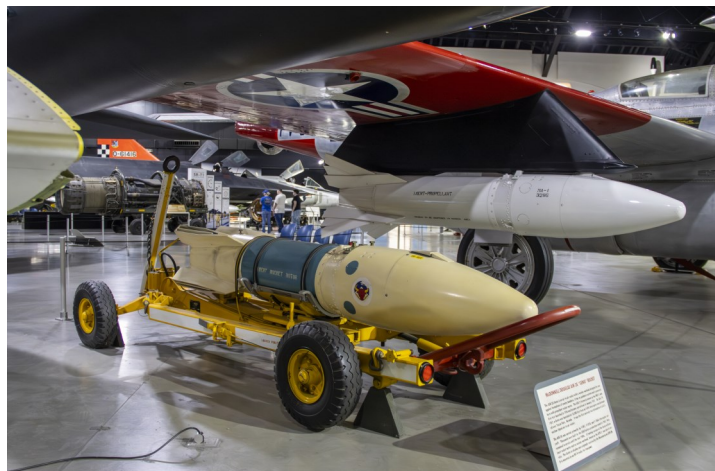
MA-1 Genie air-to-air rocket and inert training round
