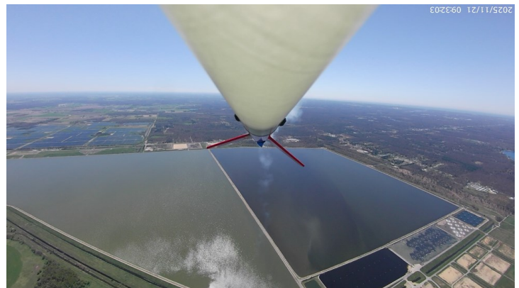
Figure 2--With the apogee charge fired at about 2500 feet, the air frame sets sail, headed due south, tail-first, with the rest of the deployed--but JLCR--restrained to 700'--recovery train in tow. (NOTE: Photo inverted for clarity.)
