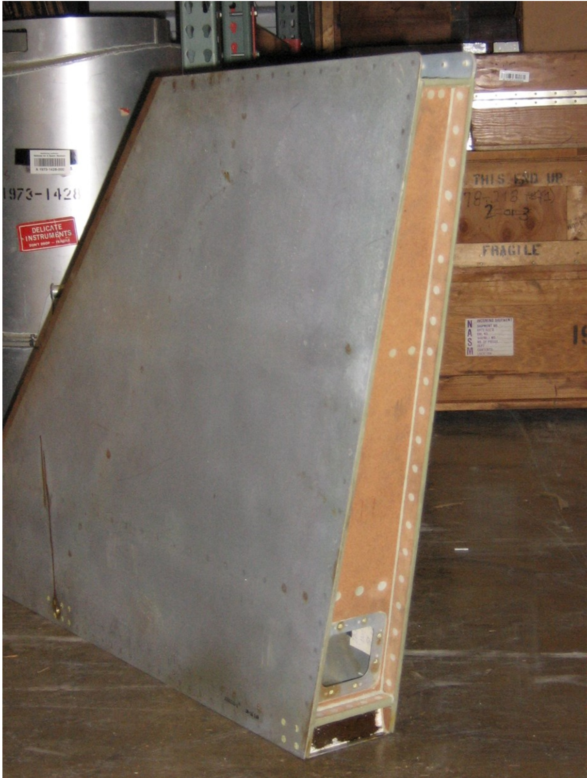
Photo 1: A350 Sustainer Fin Trailing Edge
