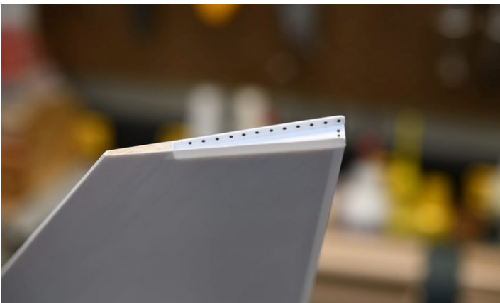
Photo 31: Tip Rivets in Place
