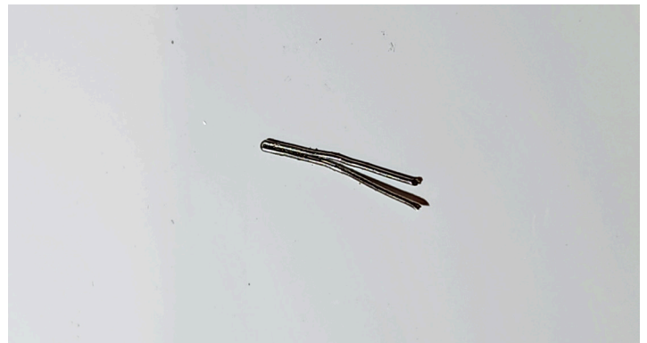
Nichrome wire cut and bent to shape before soldering
