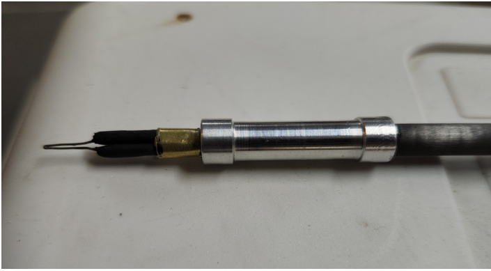
SIP Nichrome igniter in a 10mm piston
